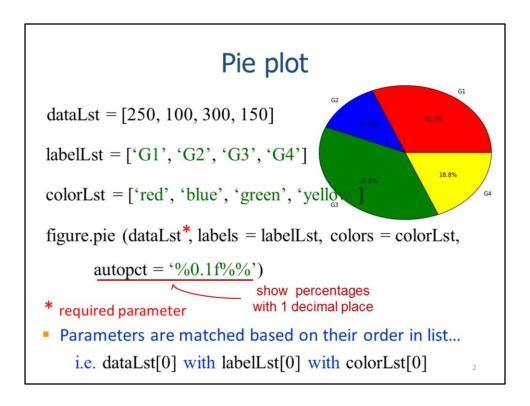
This slide will show how to create the pie plot shown here. The dataLst contains the values that will be plotted. The labelLst contains the labels that will be used for each value. The colorLst defines the wedge colors for each value.
