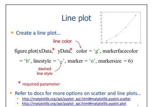
A line plot is similar to a scatter plot except that it plots sequential data such as a time series. The line plot is created using the **plot** method as shown here.
