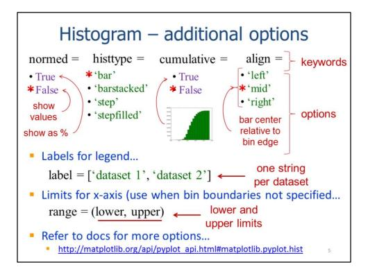
Histograms have a number of additional options – the keywords and values for a few of these options are listed here. The **normed** parameter determines if the y-axis shows absolute values or percentages. Note that asterisks indicate the default values.
